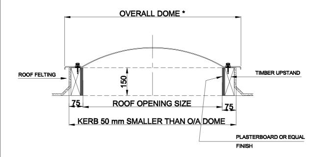
★ OVERALL DOME SIZE IS ALWAYS 200 mm LARGER THAN ROOF OPENING SIZE
