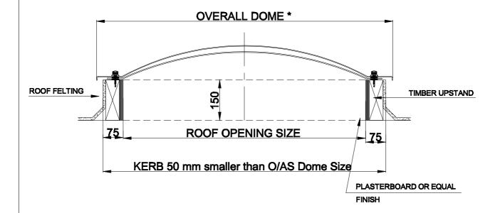
★ OVERALL DOME SIZE IS ALWAYS 200 mm LARGER THAN ROOF OPENING SIZE
